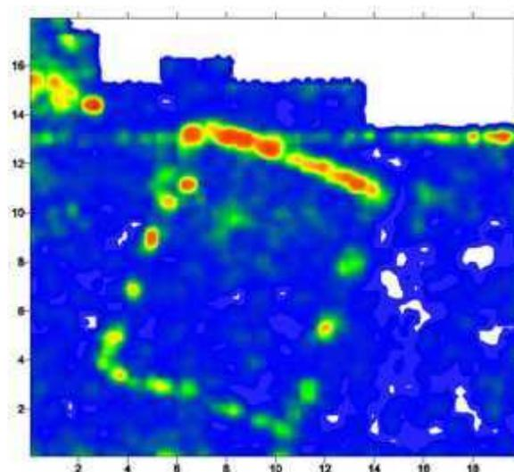
Fig.1. Amplitude Slice Map 100-150 cm. under the surface demonstrating foundations of a building and a possible Roman water line (up) by (Conyers et al., 2004).
