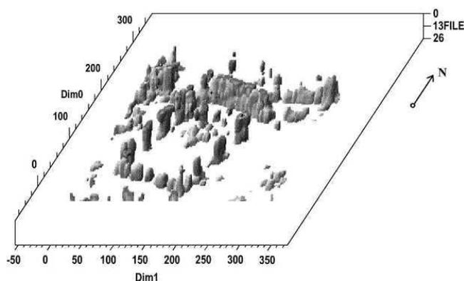
Fig.2. Three- Dimensional Rendered Surface of the foundations of the building on fig.1 constructed from Amplitude Slice Maps like this on fig.1 from various depths under the surface. (Conyers et al., 2004). Even separate stones are visible.
