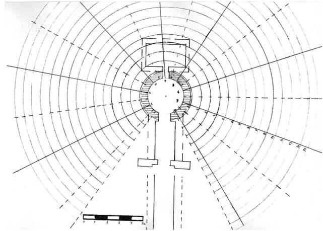
Fig. 6. Scheme of the tomb, distribution of the radar radiation during its scanning and positions of the 15 slices of 20 nanoseconds each (corresponding to a thickness of 75 cm if the radar beam passes through soil but to 3 m through air). It was unusually complicated because all important scans are vertical due to the great depth of the tomb, which makes impossible to measure it from the surface of the mound by GPR .
