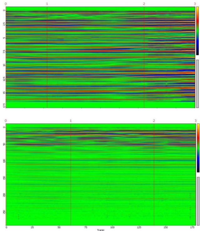
Fig. 7.A (up) A scan of the walls of the vestibule of the tomb 0- 50 cm above the floor suggesting that the radar radiation penetrates through homogeneous material at least 16 meters in all directions. Fig. 7.B (down) A scan of the walls of the vestibule of the tomb 200- 250 cm above the floor. It demonstrates that the radar radiation penetrates through the granite wall of the tomb in the homogeneous soil filling of the mound outside the tomb wall.
