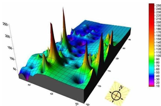
Fig.9 Map of the electric resistivity of Omurtag tomb. Vertical axis is in units of Ohm/m. (Shopov, 2007)
