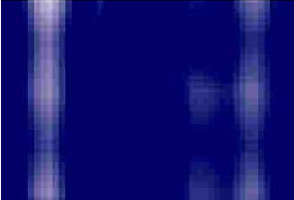
**2D map (in meters) of the radar signal of two concrete girders in the middle of the ceiling of the basement of the building B of the Physics Department measured from 17 meters above, from 5 floor through 5 concrete slabs with a total thickness of 3.25 m ! This depth is with 70% greater than the manufacturer's claimed maximum working depth of the device !!!**
