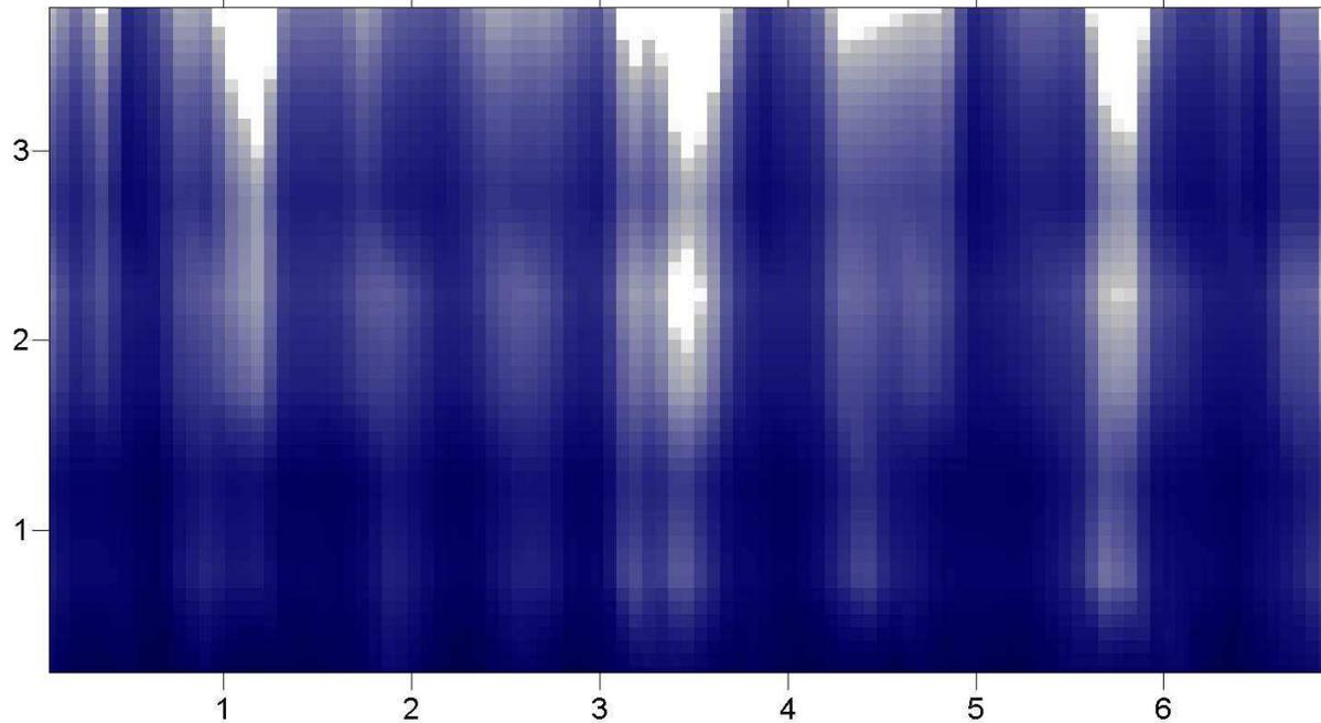
**2-D map (in meters) of the radar signal from concrete girders measured from the 5th floor of the Physics Department through the concrete floor above them. Even fluorescent lamps are visible between 3-4 and 4-5 meter scan!**
